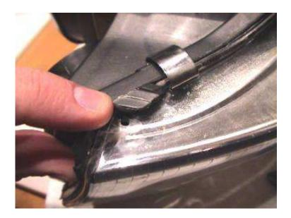
12. Use a small piece of metal (I used a small hex wrench) to push on the edge of the tab to the point where it breaks. This will now free the reflector and allow it to move within the assembly. Remove the turn signal bulb by twisting and then pulling it out. This will serve as the hole to remove the reflector.
