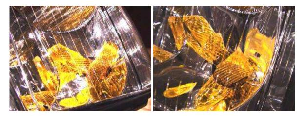
14. Using some auto silicone sealant, fill in the hole you just drilled. Don't put too much in. Put just enough in so that it spreads a tad beyond the hole. Then put a little on the outside of the hole. This will hold it anchor it to both sides of the hole. Now, put a piece of tape over the outside to hold the silicone in place and quickly turn the housing right-side up to prevent the silicone from continuing to go into the housing. Put the turn signal bulbs back in.
