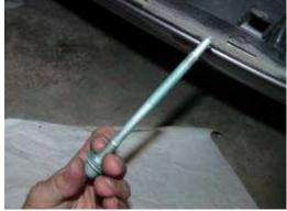
4. There is a noise insulation panel that covers the front under-side of the car. It goes from the bumper back to the transmission and out to the wheel wells. It is held in place by quick release screws/fasteners (A) on the underside of the car. It is also has plastic fasteners (B) in the front of the wheel wells. These only require a 1/4 to S turn. Remove the cover and set aside.
