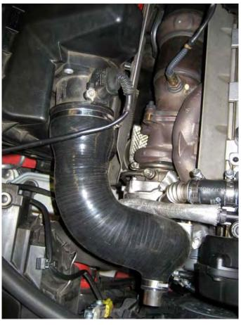
Use the supplied compressor outlet pipe and hose clamps during reassembly.
