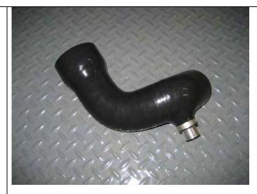
Use the supplied turbocharger inlet pipe and hose clamps during reassembly.
