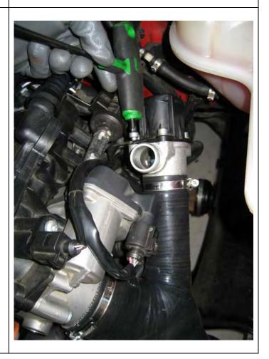
100 Connect the supplied electrical harness extension to the Turbocharger Recirculation Valve N249. 101 Attach the supplied harness clip to the EVAP hose next to the Turbocharger Recirculation Valve (N249).
