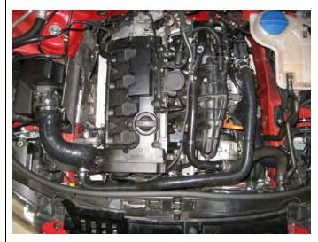
Open the bleeder bolt on the upper coolant pipe above the intake manifold. Add coolant/water mix to Coolant Reservoir until the system is at max line. Let the system degas and top off again until fluid comes out of the bleeder bolt. Close bleeder bolt and top off coolant reservoir.
