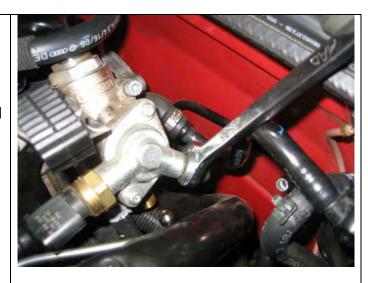
Using a T-30-Torx, remove the three bolts which retain the high pressure fuel pump to the cylinder head. Remove the bolts gradually in a sequential order.
