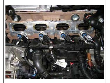
Install supplied Turbocharger Recirculation Valve N249 support bracket onto the intake manifold. Remove the two T-30-Torx bolts which support the vacuum line from the EVAP Canister Purge Solenoid Valve N80 as it heads towards the Throttle Valve Control Module J338. This step is best performed prior to reinstallation of the intake manifold.
