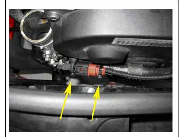
Attach one zip tie holding the harness to the coolant pipe near the spring clamp for the hose to the hard pipe
