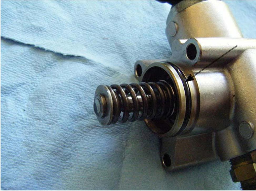
17. Time to put a new cam follower in place. Audi part number for the cam follower (sleeve) is 06D 109 309 C. It cost me \$43.20 from dealer. Carefully place the new follower into the pump opening.
