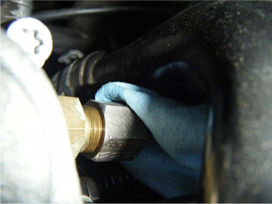
The fitting is off and the line is out of the pump fitting:
