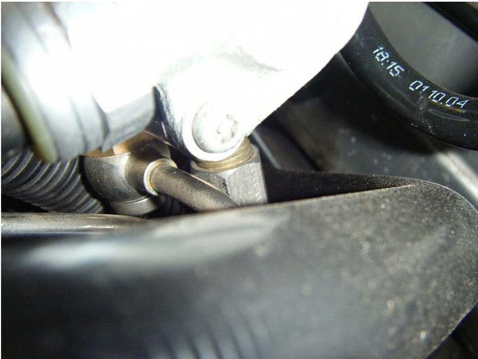
9. First, remove the high pressure line. Make sure to stuff a paper towel/work rag underneath the fitting to catch any fuel spray and drips. Use a 17mm open wrench. Suggestion: use a short wrench so that you can easily maneuver it under the coolant line, electrical wires and hoses. The fitting isn't too tight so the force applied to twist it is minimal.
