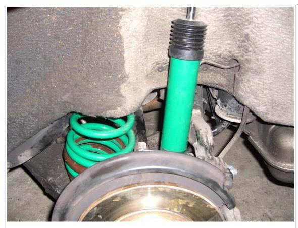
The rest is the reverse of removal. Use a jack underneath the rear hub to raise or lower everything as necessary to align bolt holes.
