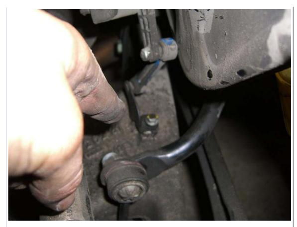
Next, remove the two 14mm bolts holding the upper shock mount on. Pull away the fender lining and use a long extension to get up there.
