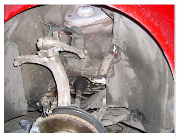
Now, remove the lower strut mount bolt (18mm). Once this is removed, finagle the whole strut assembly out.
