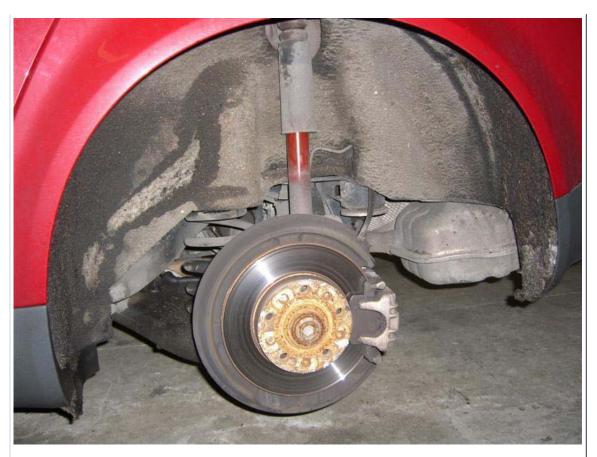
Remove the rear caliper. It is held on by two 13 bolts, but you will need a 15mm wrench for the backing bolt to keep it from turning. Tie the caliper out of the way with a piece of string or a zip tie.
