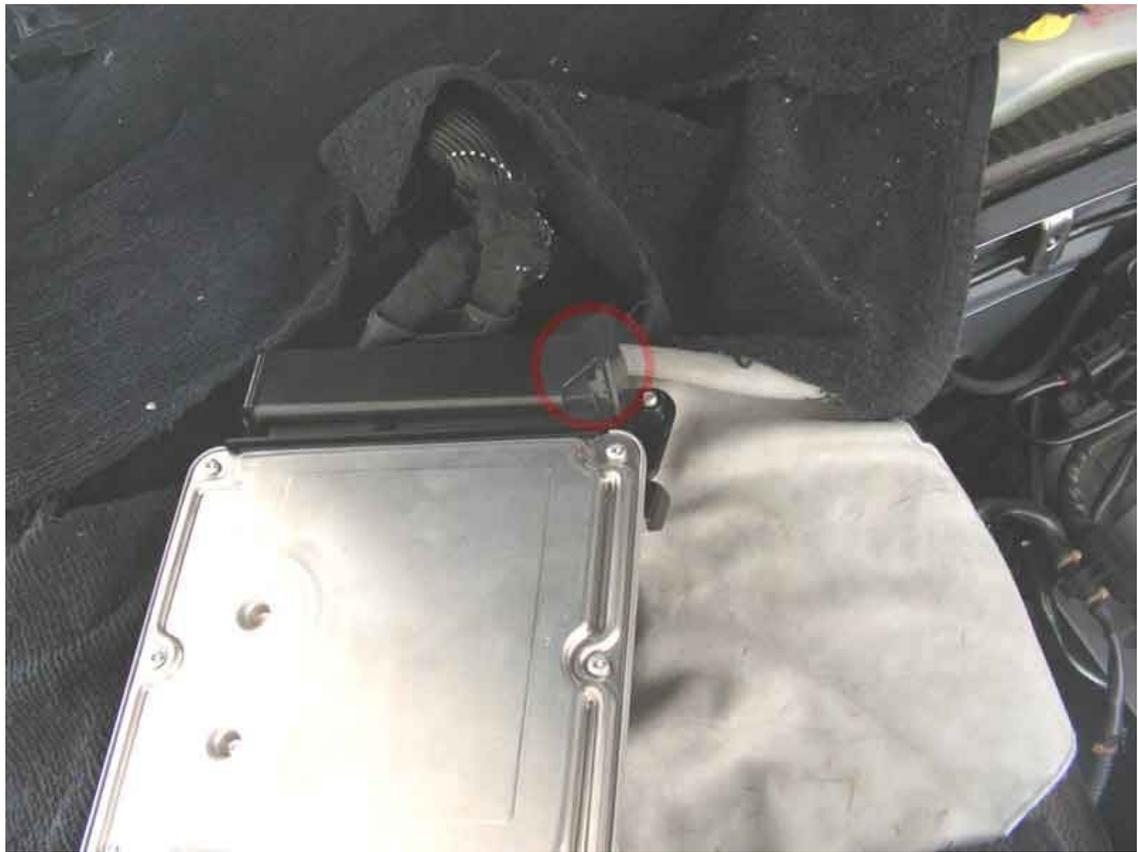
Once cut we just expand the bracket and peel it off the ECU connectors.
