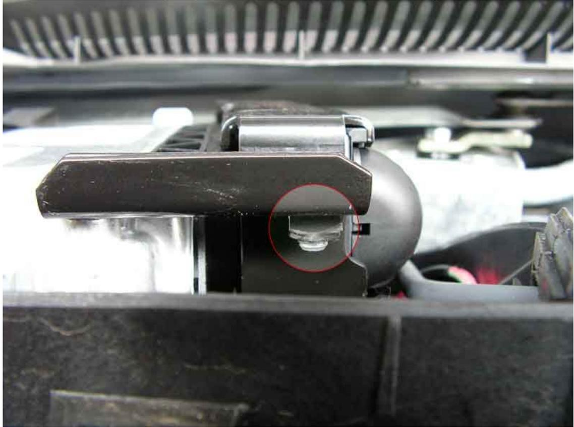
Once the screws are removed separate the two bracket pieces which uncover the ECU connectors. Unplug the connector (by pulling a small flap outward on each side) and your done.
