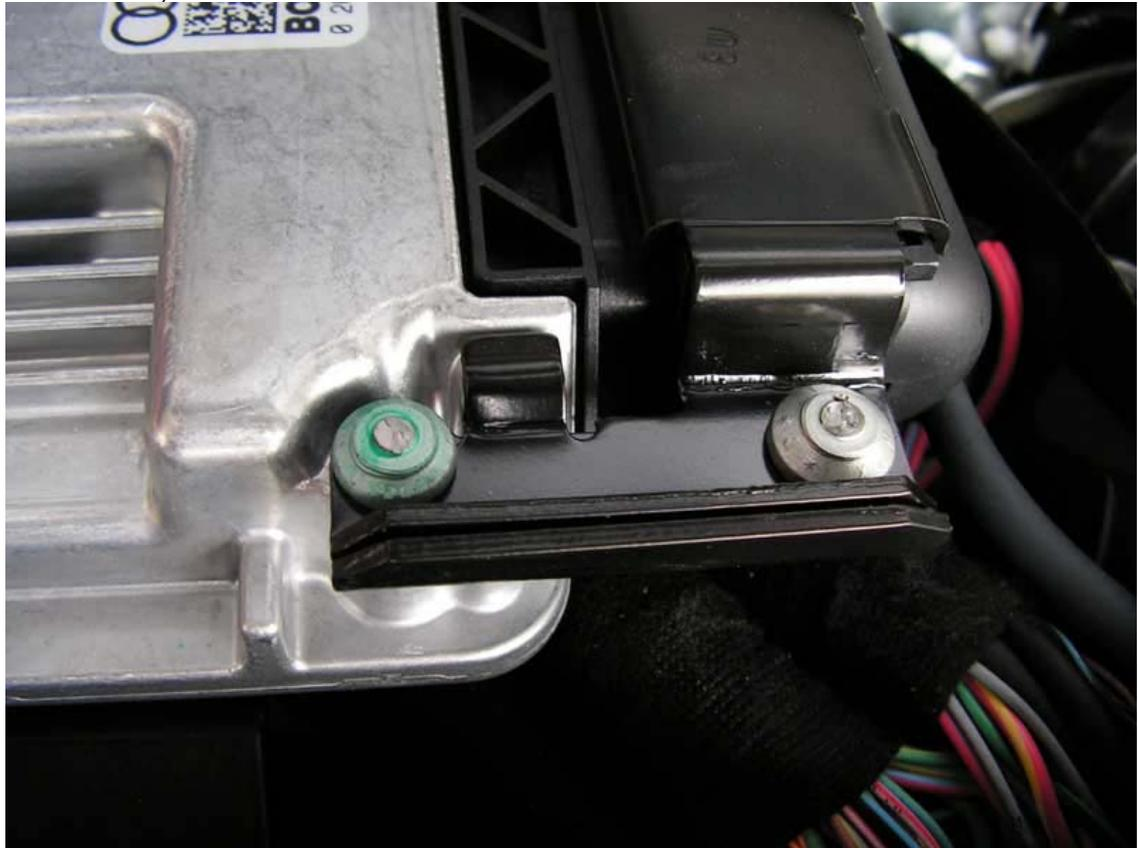
To remove the green security bolts just get the dremel out and cut a slot into them.
