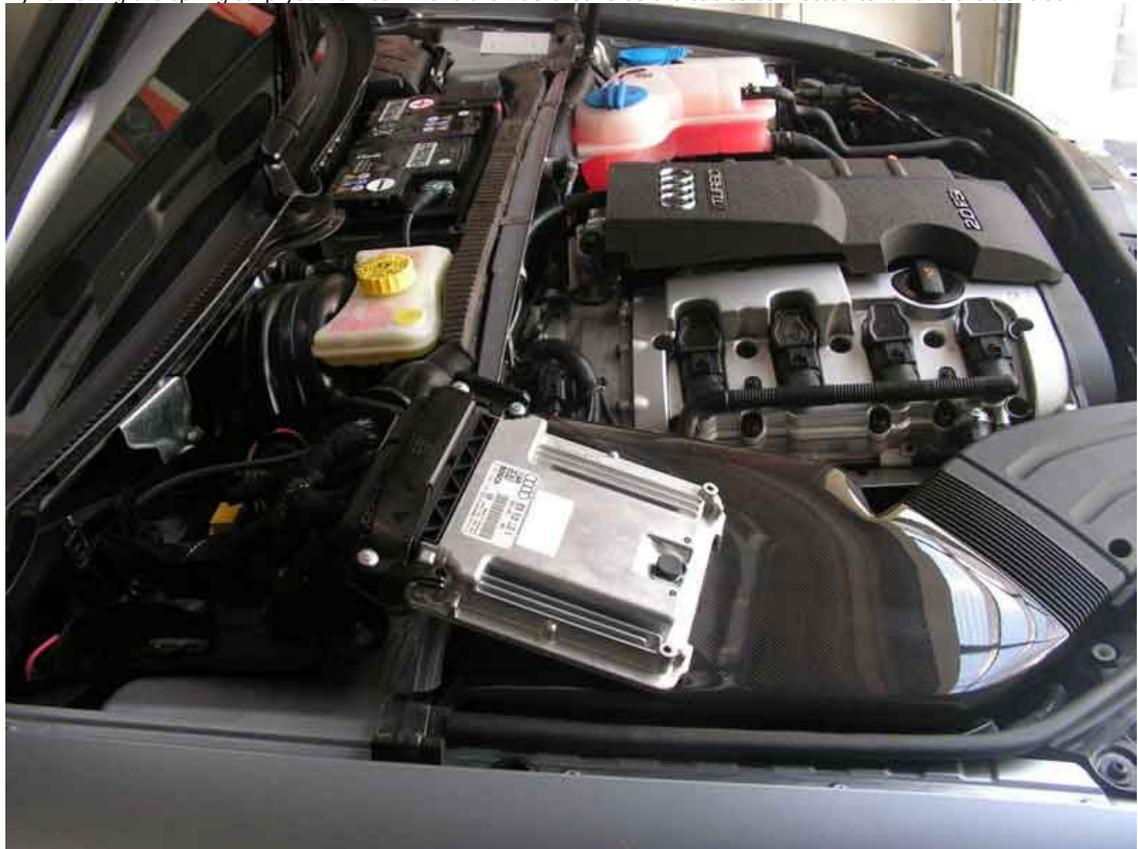
Two of the security bolts (Green ones) that are connected to the ECU can be removed with ease. The other two have
