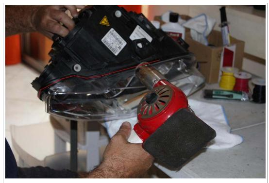
Now, grab two rags, hold the headlight vertically and separate the lens from the housing. The lens shape on the turn signal side provides a good grip. If it's too hard to pull, you can heat up a bit more the area.
