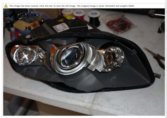
Now you need to remove the internal housing. There are 3 screws holding it in place. Location materialized in red
