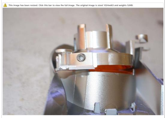
Using a razor blade, you are going to trim just a bit of the edge of the center pin, trying to make a chamfer.
