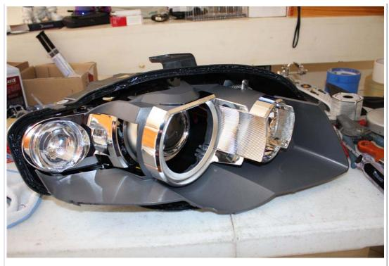
On some headlights, it's a bit more difficult because the housing stays clipped in the turn signal area. Gently pry under the plastic tab to release it. Here is a close up of the tab that may stay clipped
