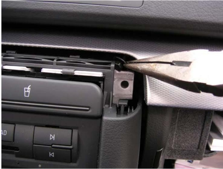
The whole thing pulls out straight. You may need to tilt the bottom of the trim upwards and wiggle it.
