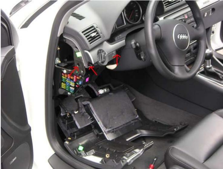
There are 3 bolts holding the trim in place (marked above). To remove these you need your new best friend, a 5/16ths socket with a screwdriver attachment and a socket wrench.
