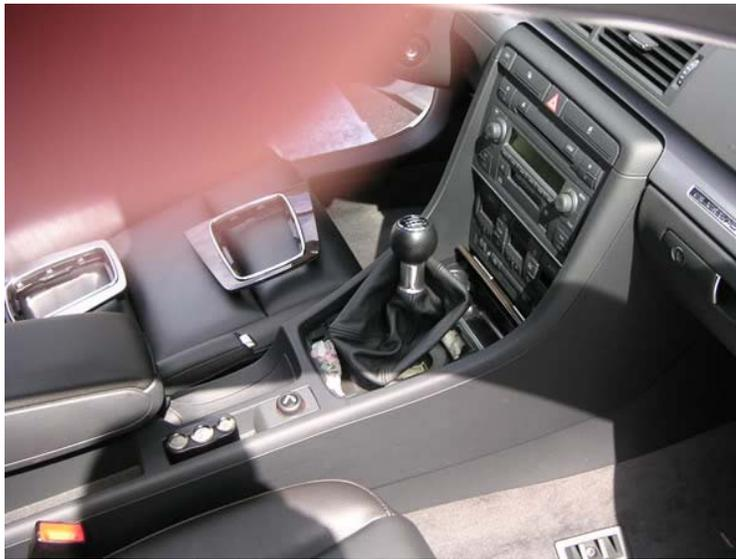
The trim piece just pulls straight up. It is secured by 4 little clips that fit into holes like the one below.
