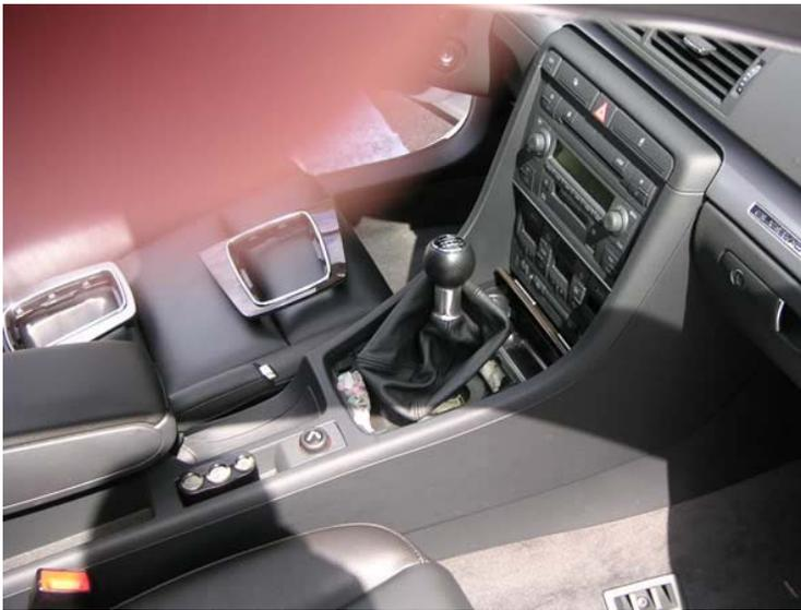
The trim piece just pulls straight up. It is secured by 4 little clips that fit into holes like the one below.
