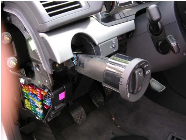
The lighting assembly of course has a few wires plugged into it. So too does the interior light dimming switch just to the right. Both can be easily unplugged and the unit themselves pushed through the trim (away from the dash). Once those are free, just put the lighting pieces into the new trim and re-secure everything. Do not put the lower dash back yet as you will need to access one of the bolts it covers when you replace the next trim piece.
