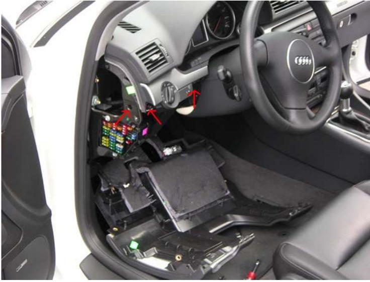
There are 3 bolts holding the trim in place (marked above). To remove these you need your new best friend, a 5/16ths socket with a screwdriver attachment and a socket wrench.
