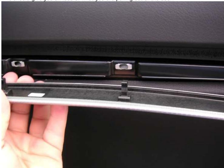
When you get to the end, the final clip slides out in the direction of the door hinge. Just simply push it towards the hinge and it will pop right out. The two rear doors have enough of an overhang that you do not need to use the screw driver to get them going. Just use your fingers to get the first one going.
