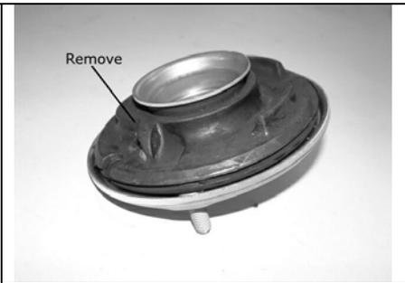
17. Install the [shock shaft load-distributing washer](#), followed by the [upper spring perch rubber bushing](#) on the threaded part of the shock shaft (\*Note\* there are two indents on the [rubber bushing that need to line up with the bolts on the upper spring perch](#)).
