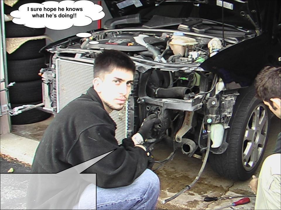
Since the IPP ICs are much larger than OE, the fender mounting bolts must be temporarily removed, to allow the core to slide into place.
