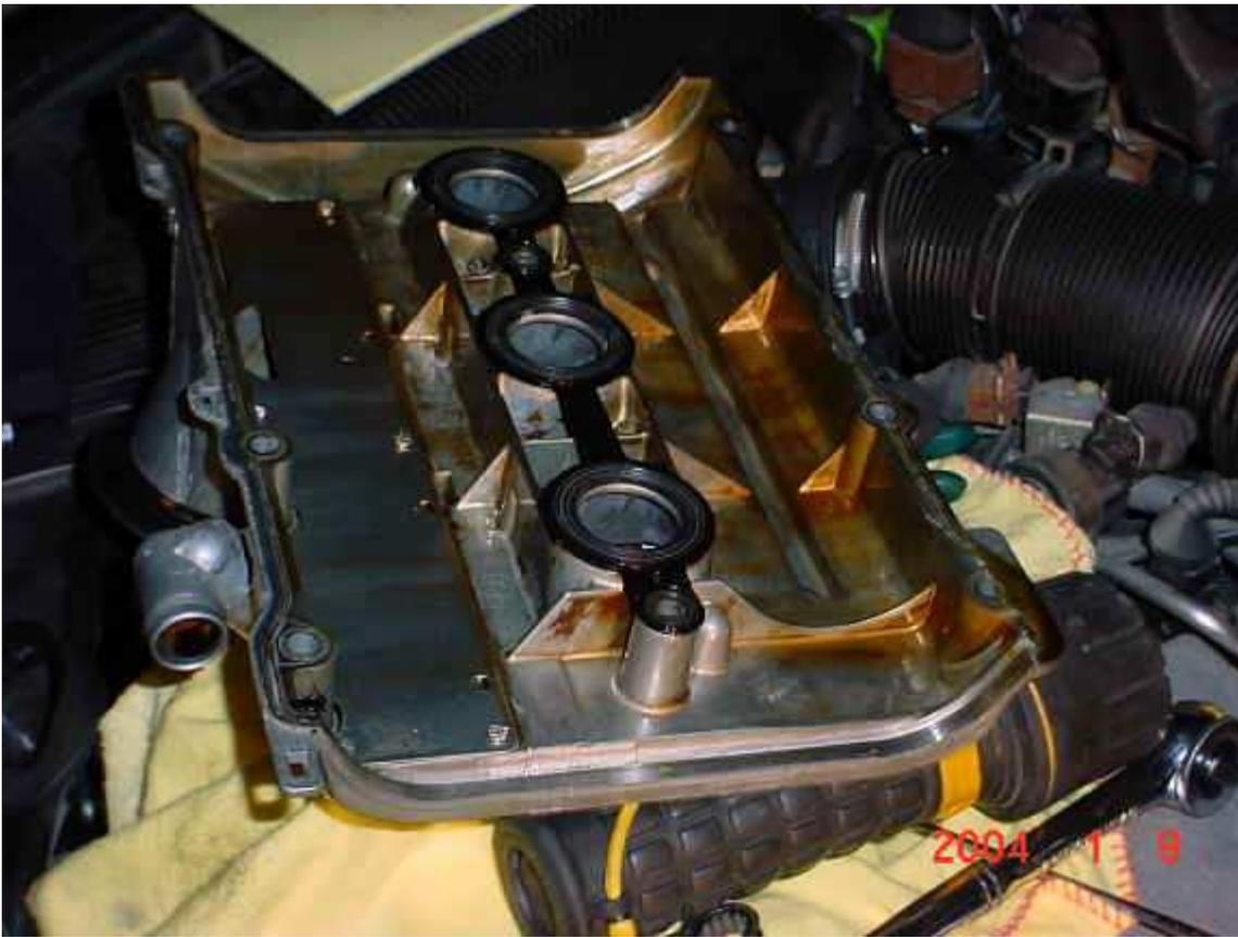
Above you can see the second portion of the gasket (center gasket). Remove this gasket and again clean up the outer and center surfaces with brake cleaner and a rag.
