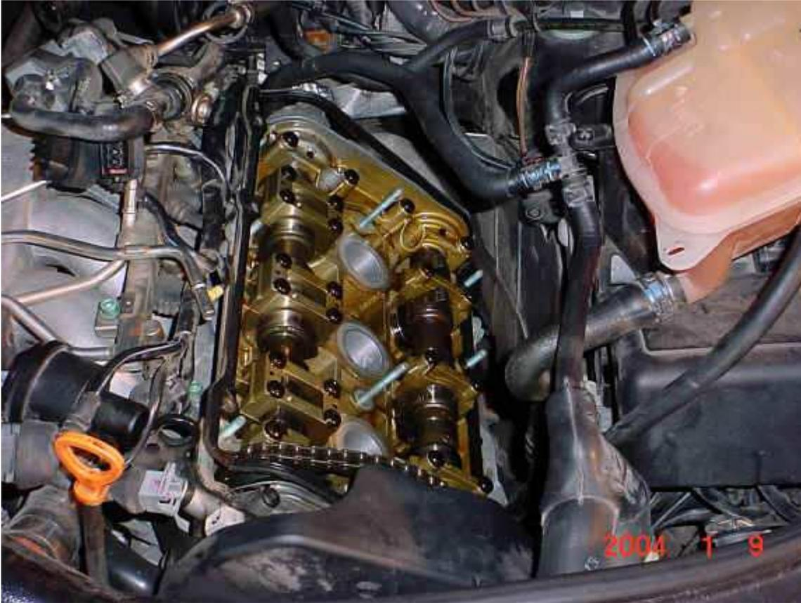
In the picture above, you can see one piece of the old gasket around the outside of the head (outer gasket). Remove the gasket and clean the surface of the head with brake cleaner and a rag. Also, clean around the spark plug holes and bolts. Make sure all debris is cleaned from the surface of the head.
