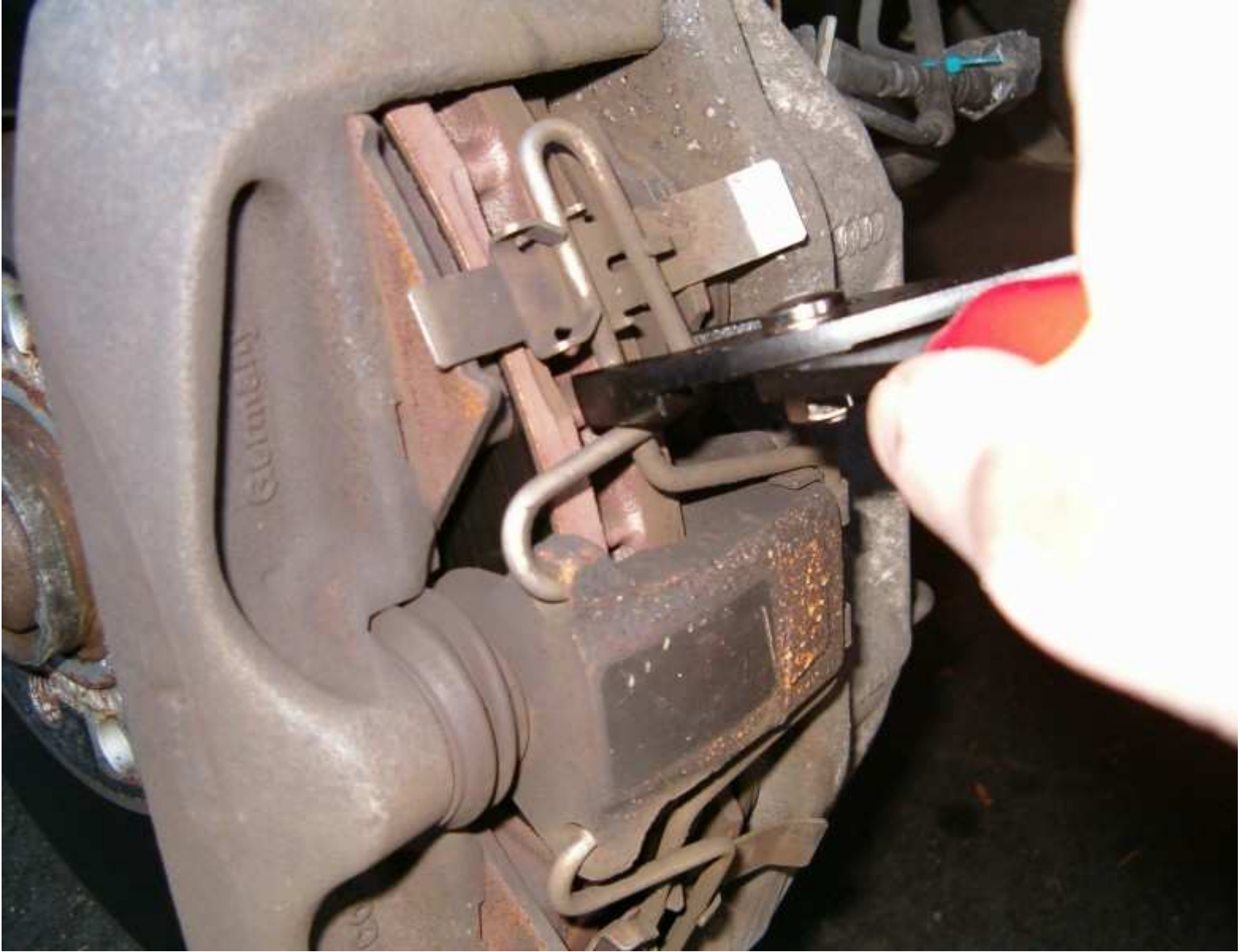
5. Hook coming out of hole when squeezing
