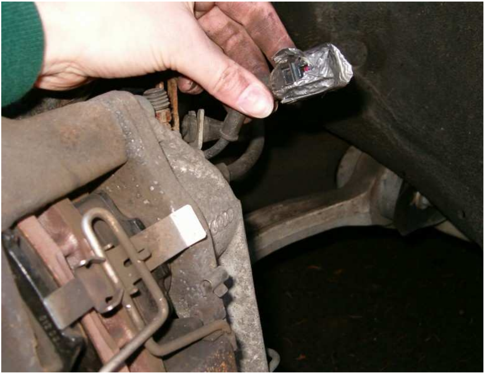
14. Example of little wire I use to short the sensor when not using stock pads.
