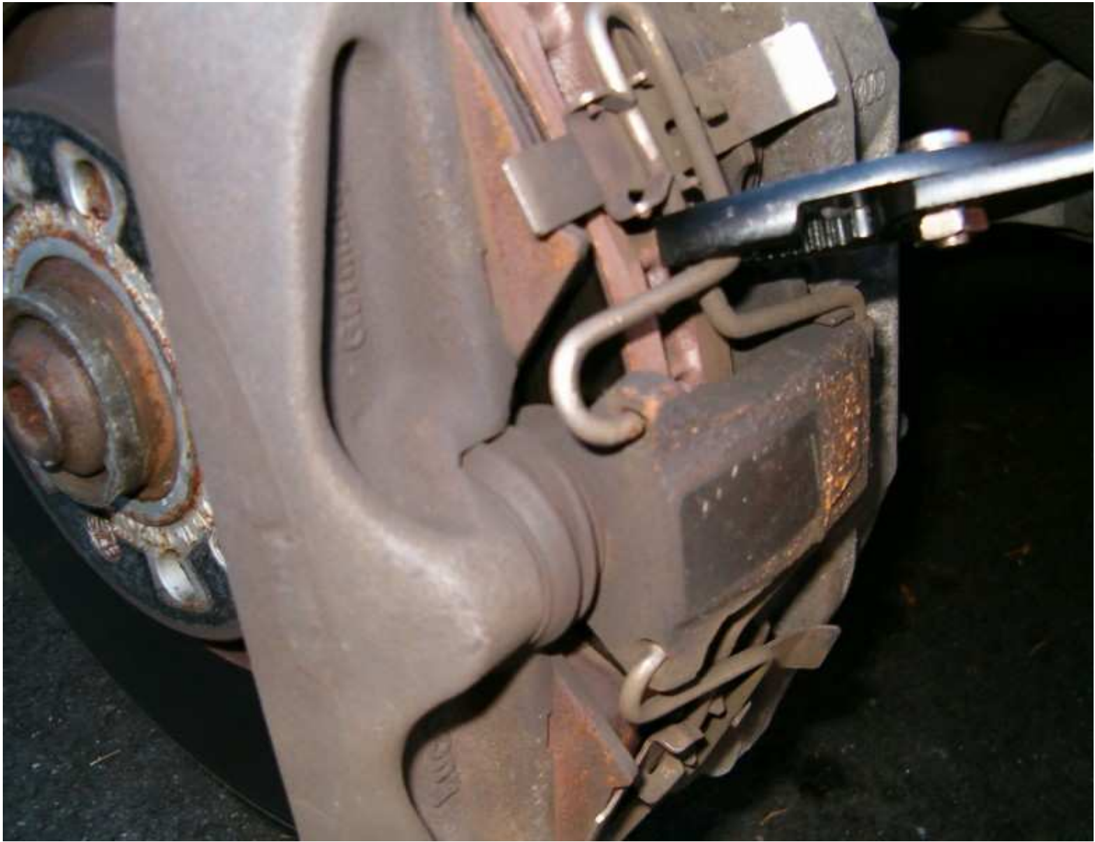
6. Unhook both top and bottom clamps
