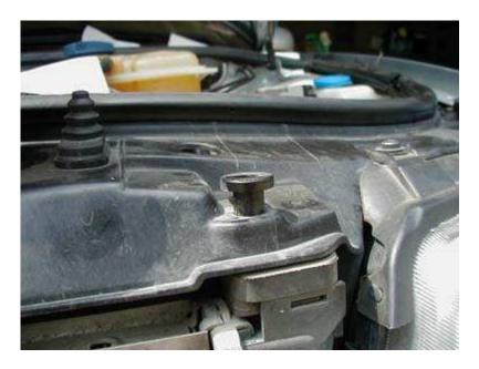
9. Now pull the top of the radiator out towards you (as if the bottom edge were a hinge), then up. The radiator is now free. Its a good idea to flush the radiator out with a garden hose at this time and let it dry while finishing up with the rest of the tbelt change
