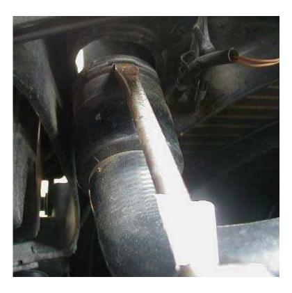
Do this for the top and bottom hoses. Now, just pull firmly (read: HARD) to get the hoses off. See the sensor above the lower radiator hose in the picture below
