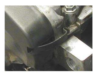
2. Remove the viscous fan; have someone hold the plastic blades firmly, while you remove the 5mm hex bolts, circled in yellow.
