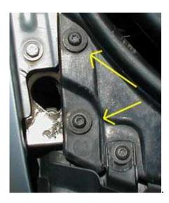
5. Remove one Torx T30 bolt underneath each headlight; see green arrow.
