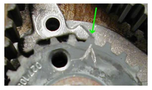
8. Remove the old tensioner and pulley. First remove 13mm the bolt holding the "guide pulley" (that's what we'll call it) on to the tensioner (green arrow); remove this pulley--save it. Now remove the two 10mm bolts holding the tensioner to the block (red arrows). Remove the 10mm nut holding the pulley on (as circled in yellow,
