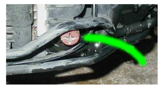
2. Disconnect the upper and lower radiator hoses, as well as the sensor just above the lower radiator hose. First, pry up the clip around the radiator fitting with a flathead screwdriver:
