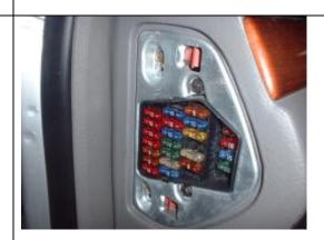
Tap fuse location number# 7, remove 5 amp fuse, and add 5 amp fuse with power led.
