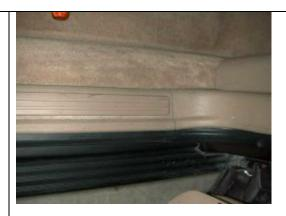
STEP 2: Remove the three Phillips screws that hold the door sill trim in place
