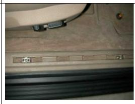
STEP 3: Move the door sill trim so that it clears the edge of the kick panel trim. Pry open the small circular plastic cover (not shown in photo) on the kick panel and remove the Phillips screw. Then pull the kick panel out and away from the door jamb (where it is held in place with metal clips.
