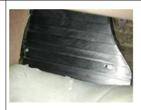
STEP 5: The Bosch Motronic ECU is held in place with four Phillips screws. Remove the screws and carefully pull the ECU up and out enough to disconnect the manifold pressure hose and the wiring harness
