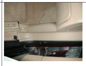
STEP 4: Remove the floor mat. Pull back on the carpet as shown. Note: the carpet and padding will need to be carefully cut along the seam that runs along the transmission tunnel.
