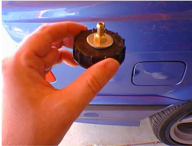
I didn't take pictures of every last little detail. Sue me. While at Pep Boys buying the cap, get a 1/4" hose fitting with a threaded base and associated brass nut. I also used a fender washer from my spare hardware bin on top. Drill a whole and enlarge to the size of the hose fitting. Screw that baby in there and secure from the back (see next pic) with the brass nut.
