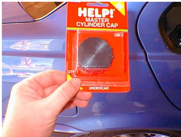
Yes its true. You can use a late model GM master cylinder cap (Help! p/n 42035). You have to take 5 seconds to modify it but it works fine after that. What you will find when you open the package is that the GM piece has a little groove cut in the underside of it to relieve pressure!?! I don't know what the hell that's about, but take some black (or whatever) RTV and using a scrap of the original packaging, smear the groove full of RTV and let it cure for a bit.
