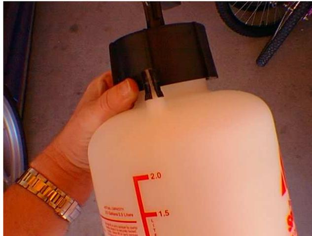
Now that you've loosened that pesky ring, cut the hose off if you can't get it to slip off. Then slit it down the side and peel it off. Set the original hose aside in case you ever want to reuse this thing as a sprayer. If so, remember to clean it *real* well first.
